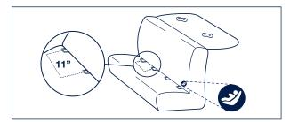
**WARNING: DO NOT USE** the **LATCH** lower anchor belts to attach this child restraint rear facing when restraining a child weighing over 35 lb (15.8 kg) or forward facing when restraining a child weighing over 40 lb (18.1 kg). Check your vehicle owner's manual for tether anchor weight limits.
