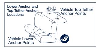
This child restraint is designed to be used with lower **LATCH** anchors at the standard spacing of 11 inches (28 cm). **LATCH** lower vehicle anchor points are defined as 11 inches (28 cm) from the center of one **LATCH** anchor to the center of another **LATCH** anchor.
