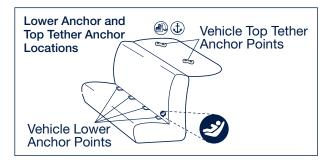
This child restraint is designed to be used with lower **LATCH** anchors at the standard spacing of 11 inches (28 cm). **LATCH** lower vehicle anchor points are defined as 11 inches (28 cm) from the center of one **LATCH** anchor to the center of another **LATCH** anchor.
