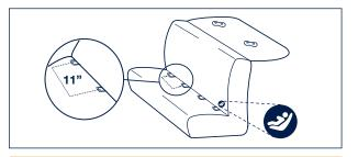
▲ WARNING: DO NOT USE the LATCH lower anchor belts to attach this child restraint rear facing when restraining a child weighing over 35 lb (15.8 kg) or forward facing when restraining a child weighing over 40 lb (18.1 kg). Check your vehicle owner's manual for tether anchor weight limits.
