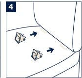
1 - Line up the Lower Anchor Connectors with the vehicle's Lower Anchors and press both connectors firmly until a click is heard and both are securely fastened.
