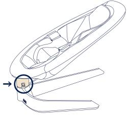
Always lock base and carry holding the seat tube when transporting.
