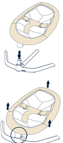
After assembly, pull up on seat to ensure it is properly secured to base.
